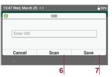
If prompted, enter, or scan the Operator ID. Select **Scan (6)** and then **Save (7)**. Wait while instrument warms and prepares cartridge.
