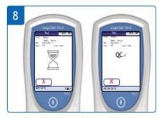
Wait for the meter to beep and start to analyse the sample then remove the finger. The meter will automatically test the on-board QC.
