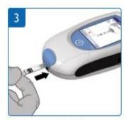
Remove a test strip from pot and insert into meter when prompted.
